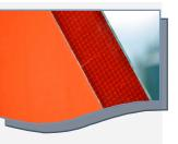
This provides an increased visibility as the marking material appears brighter. The outer red part of this SMV emblem is retroreflective while the inner orange part is a non-reflective material.
